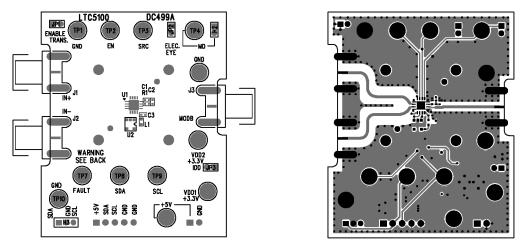
Figure 34 Layout of the DC499 Demo Board (Silkscreen and Top Layer Copper)
