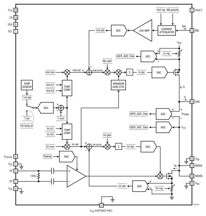
Figure 3. Functional Diagram—Automatic Power Control Mode
