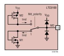
Figure 9. Equivalent Circuit for the MD Pin
