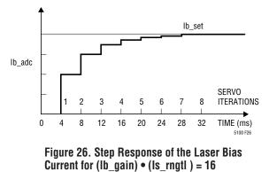
Reducing Ib\_gain slows the settling time and increasing Ib\_gain speeds the settling time. For example, with Ib\_gain  $\cdot$  (Is\_rng + 1) = 1, the residual loop error is cut by 1/32 with each servo iteration. In this case it would take 145 servo iterations (about 580ms) to settle to 1%. With Ib\_gain  $\cdot$  (Is\_rng + 1) = 31, the residual servo loop error is cut by 31/32 with each servo iteration. In this case it would take only two servo iterations (about 8ms) to settle to 1%.
