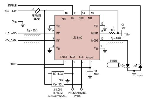
Figure 29. Schematic of a Minimum Component Count Circuit
