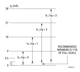
Figure 17. Ranges for the Source Current
