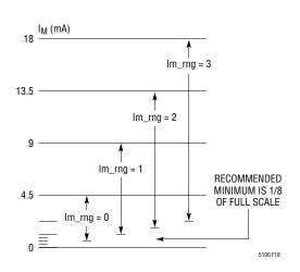
Figure 18. Ranges for the Modulation Current
