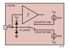
Figure 6. Equivalent Circuit for the EN Pin
