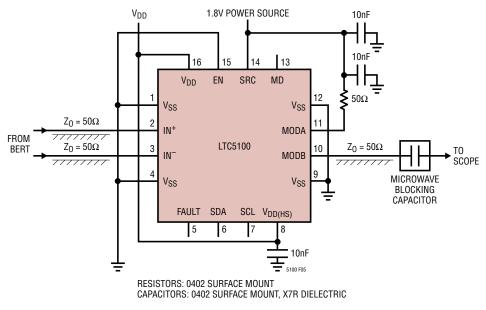
Figure 5. Test Circuit
