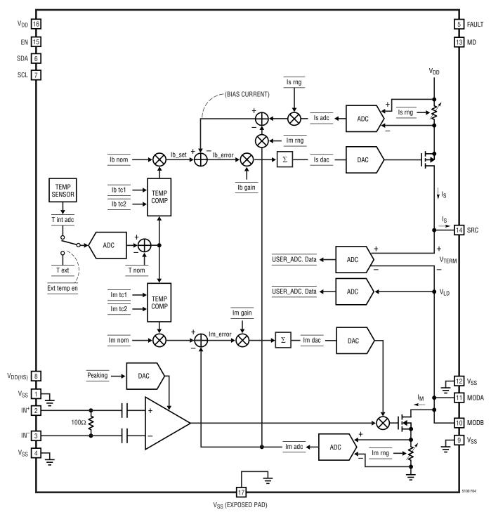
Figure 4. Functional Diagram—Constant Current Control Mode
