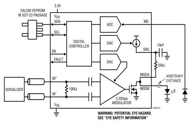
Figure 1. VCSEL Transmitter with Automatic Power Control
