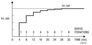
Figure 22. Step Response of the Average Modulation Current for  $\mbox{Im}_gain$  = 4
