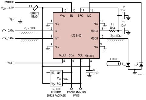
Figure 31. Schematic of a Minimum Output Reflection Coefficient Circuit
