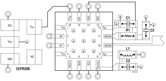
Figure 32. Layout of the Minimum Reflection Coefficient Circuit Using 0402 Passive Components
