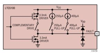
Figure 8. Equivalent Circuit for the FAULT Pin. All Switches are Open in Open-Drain Mode
