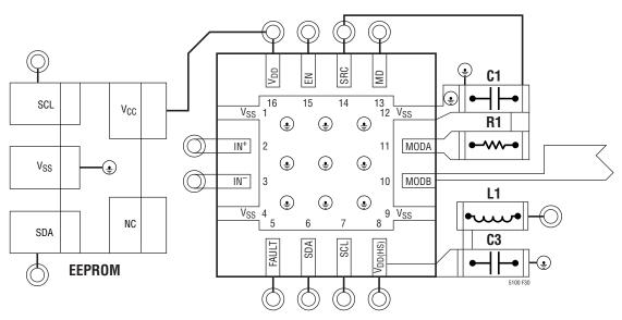
Figure 30. Layout of the Minimum Component Count Circuit Using 0402 Passive Components
