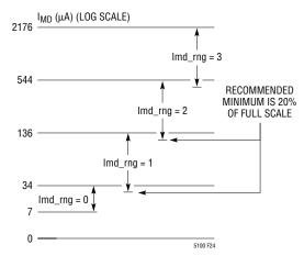
Figure 24. Operating Ranges for the Monitor Diode Current
