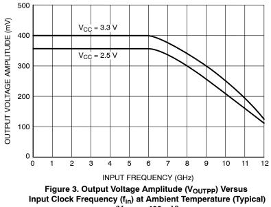
$(V_{INPP} = 400 \text{ mV})$
