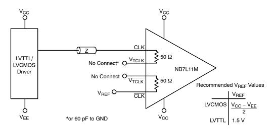
Figure 18. LVCMOS/LVTTL to CML Receiver Interface
