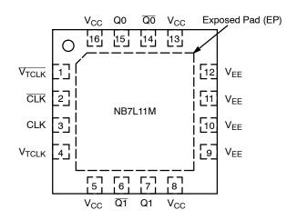
Figure 2. QFN-16 Pinout (Top View)
