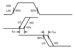
Figure 3. Delay Matching Waveform Definitions
