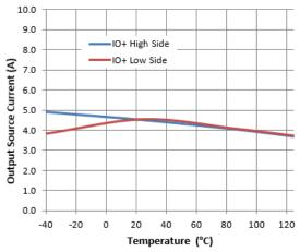
Figure 17. Output Source Current vs. Temperature
