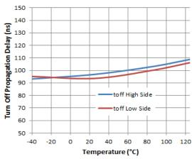
Figure 7. Turn-off Propagation Delay vs. Temperature
