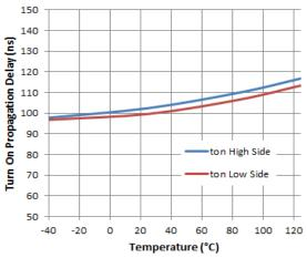
Figure 5. Turn-on Propagation Delay vs. Temperature
