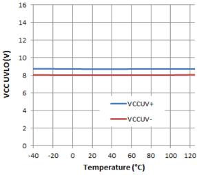
Figure 24. VCC UVLO vs. Temperature
