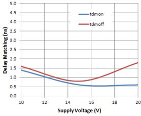
Figure 14. Delay Matching vs. Supply Voltage
