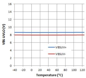
Figure 25. VBS UVLO vs. Temperature
