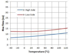
Figure 9. Rise Time vs. Temperature
