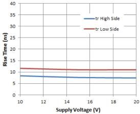
Figure 8. Rise Time vs. Supply Voltage
