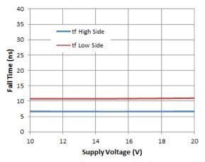
Figure 10. Fall Time vs. Supply Voltage
