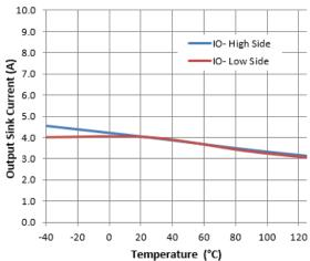
Figure 19. Output Sink Current vs. Temperature
