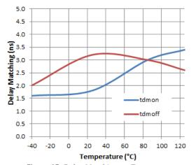
Figure 15. Delay Matching vs. Temperature
