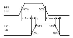
Figure 2. Switching Time Waveform Definitions
