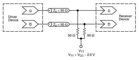
Figure 7. Typical Termination for Output Driver and Device Evaluation (See Application Note <u>AND8020/D</u> – Termination of ECL Logic Devices)
