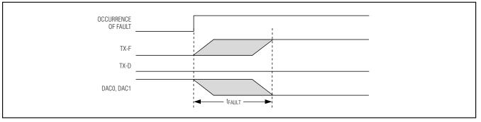
Figure 5. Detection of Transmitter Safety Fault Operation
