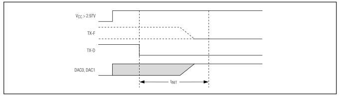
Figure 2. Power-On Initialization with TX-D Asserted
