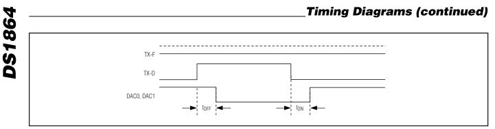
Figure 4. TX-D Timing During Normal Operation
