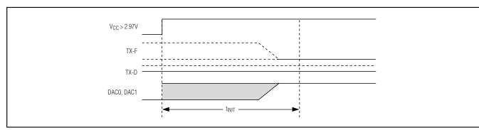
Figure 1. Power-On Initialization with TX-D Low
