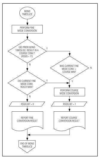
Figure 15. Dual-Range Functionality Flowchart
