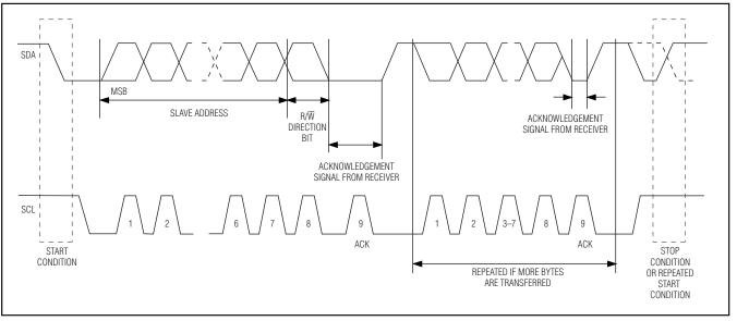
Figure 18. I<sup>2</sup>C Data Transfer Protocol
