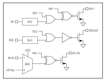
Figure 13. Block Diagram, Outputs
