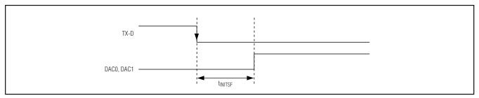
Figure 10. Output Enable/Recovery from Safety Fault Shutdown
