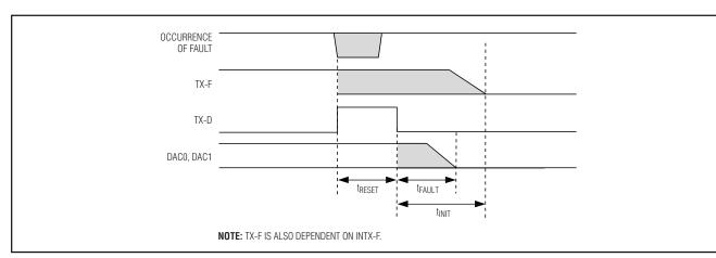
Figure 7. Unsuccessful Recovery from a Transient Safety Fault Condition
