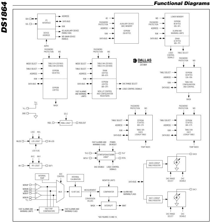
Figure 11. Block Diagram, Main
