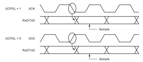
The UCPOLn bit UCRSC selects which XCK clock edge is used for data sampling and which is used for data change. As Figure 18-3 shows, when UCPOLn is zero the data will be changed at rising XCK edge and sampled at falling XCK edge. If UCPOLn is set, the data will be changed at falling XCK edge and sampled at rising XCK edge.
