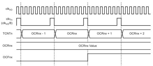
Figure 16-11 shows the setting of OCF2A and the clearing of TCNT2 in CTC mode.
