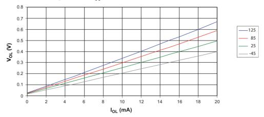
Figure 28-21. Output Low Voltage Port B - V<sub>cc</sub> = 3V
