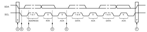
Figure 19-5. Two-wire Mode, Typical Timing Diagram
