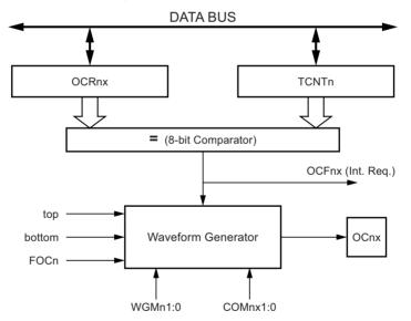
The OCR0A register is double buffered when using any of the pulse width modulation (PWM) modes. For the normal and clear timer on compare (CTC) modes of operation, the double buffering is disabled. The double buffering synchronizes the update of the OCR0 compare register to either top or bottom of the counting sequence. The synchronization prevents the occurrence of odd-length, non-symmetrical PWM pulses, thereby making the output glitch-free.
