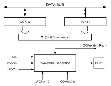
The OCR2A register is double buffered when using any of the pulse width modulation (PWM) modes. For the normal and clear timer on compare (CTC) modes of operation, the double buffering is disabled. The double buffering synchronizes the update of the OCR2A compare register to either top or bottom of the counting sequence. The synchronization prevents the occurrence of odd-length, non-symmetrical PWM pulses, thereby making the output glitch-free.
