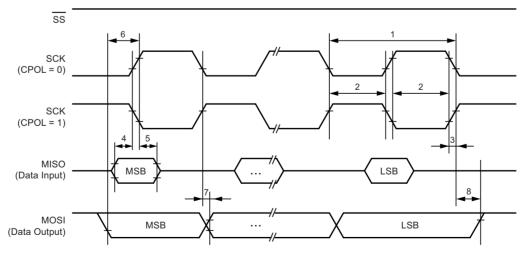
Figure 27-4. SPI Interface Timing Requirements (Slave Mode)
