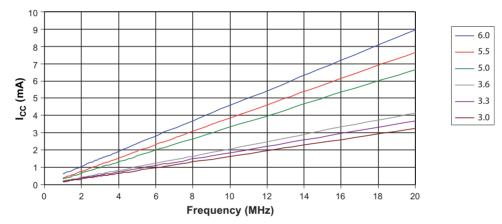
Figure 28-7. Idle Supply Current versus  $V_{CC}$  (Internal RC Oscillator, 8MHz)
