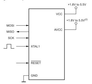
Note: 1. If the device is clocked by the internal oscillator, it is no need to connect a clock source to the XTAL1 pin.
