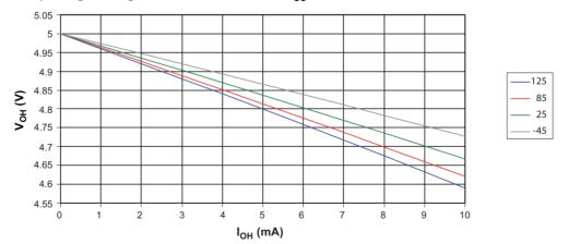
Figure 28-23. Output High Voltage Ports A, C, D, E, F, G - V<sub>CC</sub> = 3V
