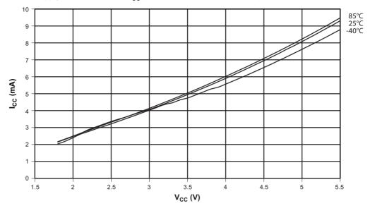
Figure 28-4. Active Supply Current versus V<sub>CC</sub> (Internal RC Oscillator, 1MHz)
