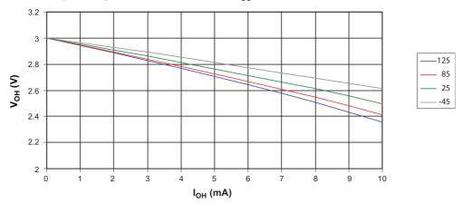
Figure 28-24. Output High Voltage Port B -  $V_{CC} = 5V$
