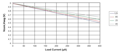
Figure 28-27. LCD SEG Output Buffer Impedance
