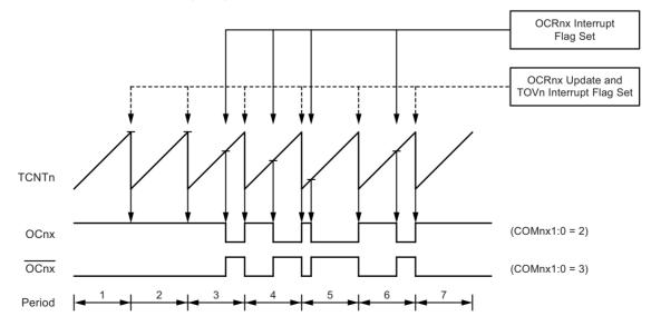
The timer/counter overflow flag (TOV2) is set each time the counter reaches MAX. If the interrupt is enabled, the interrupt handler routine can be used for updating the compare value.
