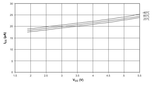
Figure 28-36. ADC Current versus  $V_{CC}$  (AREF = AVCC)
