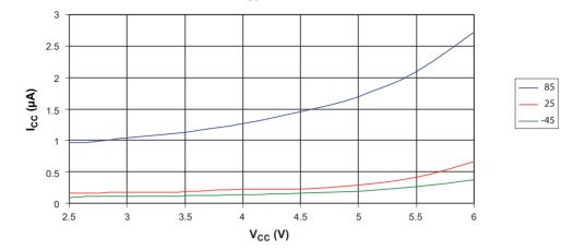
Figure 28-9. Power-down Supply Current versus V<sub>CC</sub> (Watchdog Timer Disabled)
