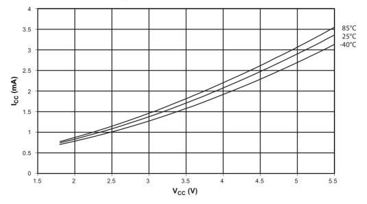
Figure 28-8. Idle Supply Current versus V<sub>CC</sub> (Internal RC Oscillator, 1MHz)
