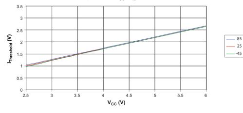
Figure 28-16. Reset Input Threshold Voltage versus V<sub>CC</sub> (V<sub>IH</sub>, Reset Pin Read as "1")
