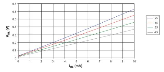
Figure 28-19. Output Low Voltage Ports A, C, D, E, F, G - V<sub>CC</sub> = 3V
