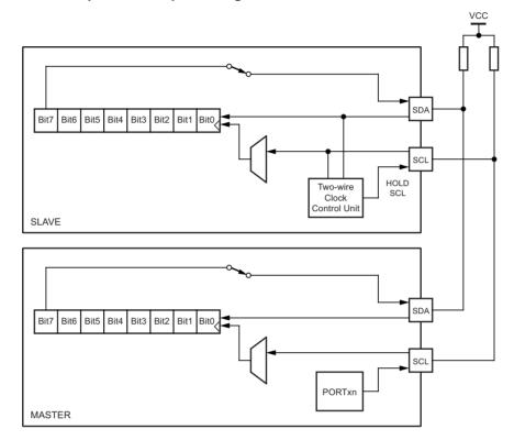
Figure 19-4. Two-wire Mode Operation, Simplified Diagram
