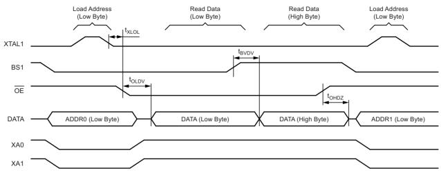
Note: 1. The timing requirements shown in Figure 26-7 on page 262 (i.e., t<sub>DVXH</sub>, t<sub>XHXL</sub>, and t<sub>XLDX</sub>) also apply to reading operation.
