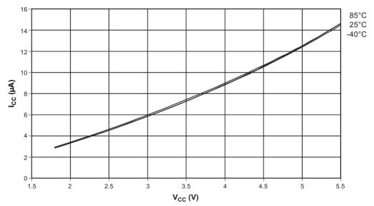
Figure 28-39. Analog Comparator Current versus V<sub>cc</sub>
