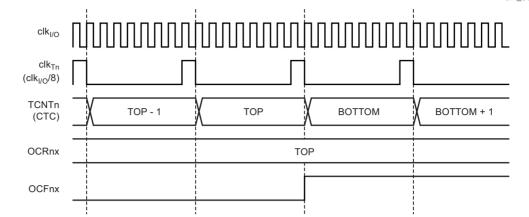
Figure 16-11.Timer/Counter Timing Diagram, Clear Timer on Compare Match mode, with Prescaler (f<sub>clk I/0</sub>/8)
