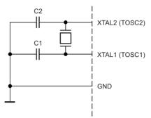
The oscillator can operate in three different modes, each optimized for a specific frequency range. The operating mode is selected by the fuses CKSEL3:1 as shown in Table 7-5.
