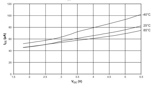
Figure 28-40. Programming Current versus  $V_{CC}$
