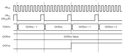
Figure 14-12 shows the count sequence close to TOP in various modes. When using phase and frequency correct PWM mode the OCR1x register is updated at BOTTOM. The timing diagrams will be the same, but TOP should be replaced by BOTTOM, TOP-1 by BOTTOM+1 and so on. The same renaming applies for modes that set the TOV1 flag at BOTTOM.
