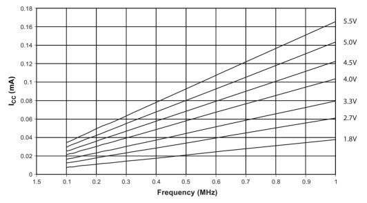
Figure 28-42. Reset Supply Current versus V<sub>CC</sub> (1 - 16 MHz, Excluding Current Through The Reset Pull-up)
