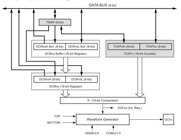
Figure 14-4. Output Compare Unit, Block Diagram
