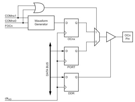
The general I/O port function is overridden by the output compare (OC0A) from the waveform generator if either of the COM0A1:0 bits are set. However, the OC0A pin direction (input or output) is still controlled by the data direction register (DDR) for the port pin. The data Direction register bit for the OC0A pin (DDR\_OC0A) must be set as output before the OC0A value is visible on the pin. The port override function is independent of the waveform generation mode.
