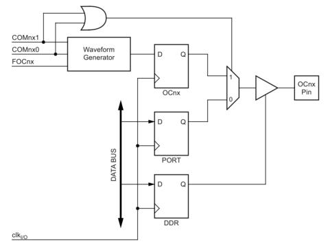
The general I/O port function is overridden by the output compare (OC2A) from the waveform generator if either of the COM2A1:0 bits are set. However, the OC2A pin direction (input or output) is still controlled by the data direction register (DDR) for the port pin. The data direction register bit for the OC2A pin (DDR\_OC2A) must be set as output before the OC2A value is visible on the pin. The port override function is independent of the waveform generation mode.
