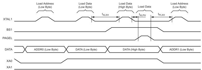
Note: 1. The timing requirements shown in Figure 26-7 (i.e.,  $t_{DVXH}$ ,  $t_{XHXL}$ , and  $t_{XLDX}$ ) also apply to loading operation.
