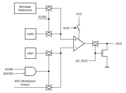
Figure 24-8. General Boundary-scan cell Used for Signals for Comparator and ADC
