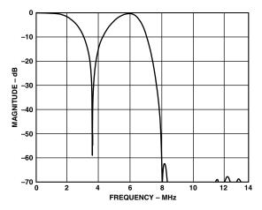
Figure 8. NTSC Notch Luma Filter
