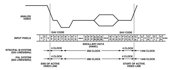
Figure 23. Timing Mode 0 (Slave Mode)
