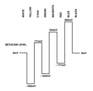
Figure 86. NTSC 100% Color Bars, No Pedestal U Levels
