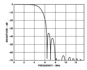
Figure 7. PAL Low-Pass Luma Filter
