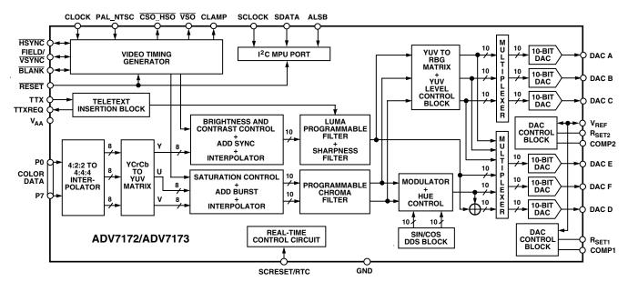
The ADV7172/ADV7173 is designed with four color controls (hue, contrast, brightness and saturation). All YUV formats (SMPTE/EBU N10, MII and Betacam) are supported in both PAL and NTSC.
