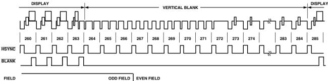
Figure 34. Timing Mode 3 (NTSC)
