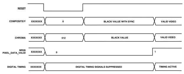
Figure 36. RESET Sequence Timing Diagram
