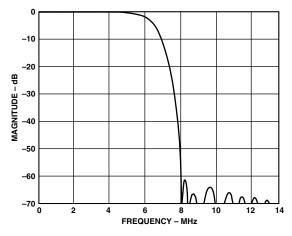
Figure 10. Extended Mode (SSAF) Luma Filter
