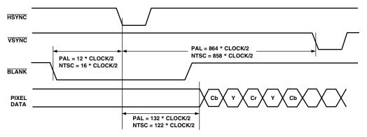
Figure 33. Timing Mode 2 Odd-to-Even Field Transition Master/Slave
