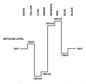
Figure 90. NTSC 100% Color Bars with Pedestal V Levels
