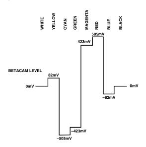
Figure 89. NTSC 100% Color Bars, No Pedestal V Levels
