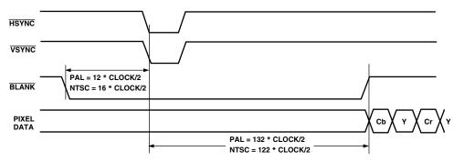
Figure 32. Timing Mode 2 Even-to-Odd Field Transition Master/Slave
