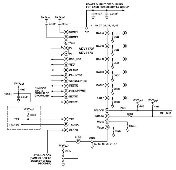
Figure 68. Recommended Analog Circuit Layout
