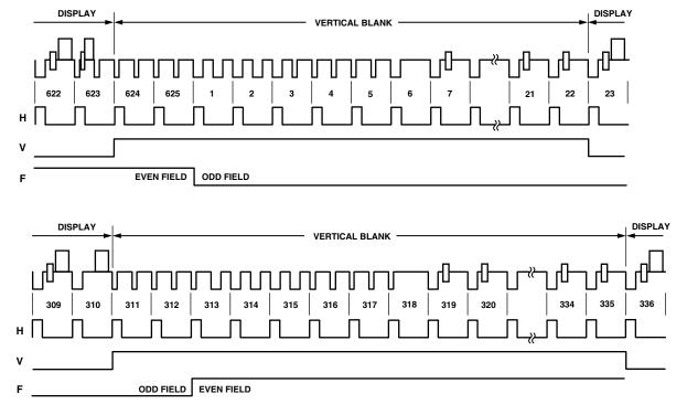
Figure 25. Timing Mode 0 (PAL Master Mode)
