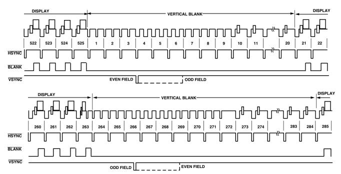
Figure 30. Timing Mode 2 (NTSC)
