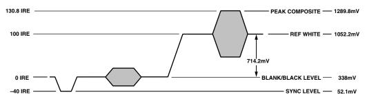
Figure 78. NTSC Composite Video Levels
