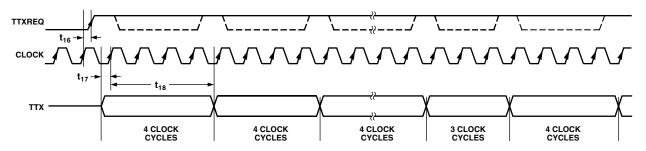
Figure 3. Teletext Timing Diagram
