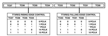
Figure 59. Teletext Request Control Register
