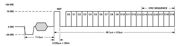
Figure 70. CGMS Waveform Diagram
