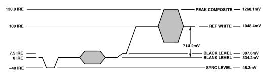
Figure 74. NTSC Composite Video Levels
