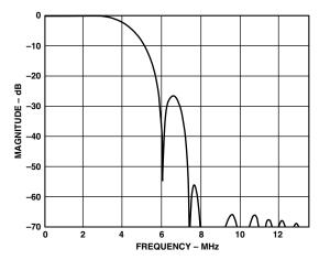
Figure 6. NTSC Low-Pass Luma Filter
