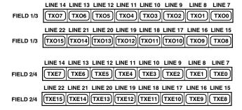
Figure 58. Teletext Control Registers
