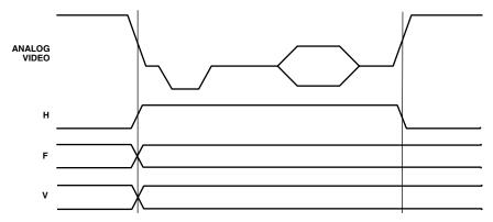
Figure 26. Timing Mode 0 Data Transitions (Master Mode)
