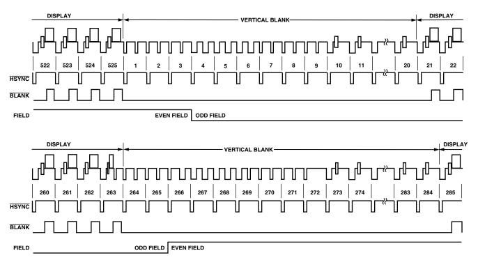
Figure 27. Timing Mode 1 (NTSC)
