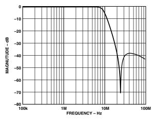
Figure 93. Output Filter Plot
