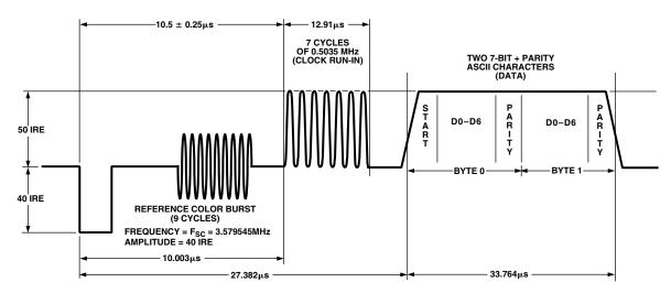
Figure 69. Closed Captioning Waveform (NTSC)
