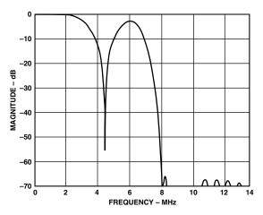
Figure 9. PAL Notch Luma Filter
