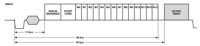
Figure 71. WSS Waveform Diagram
