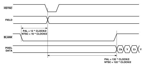
Figure 29. Timing Mode 1 Odd/Even Field Transitions Master/Slave
