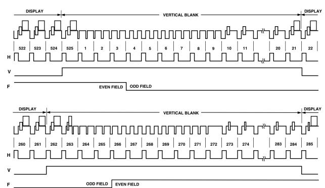
Figure 24. Timing Mode 0 (NTSC Master Mode)
